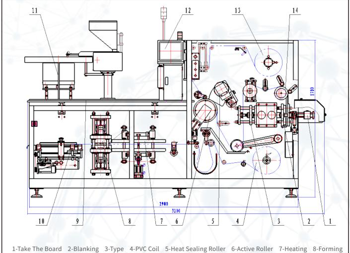
9-Platform 10-Forming step 11-Feeding 12-Touch Screen 13-Aluminum Foil Coil 14-Active Roller
