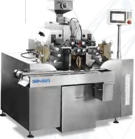
This type of machine, basically, fills the gelatin shells with semi-liquid or liquid substances. It is capable of achieving this through linear and rotary motions from different driving mechanisms including motors
