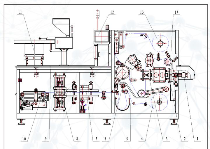
1-Take The Board 2-Blanking 3-Type 4-PVC Coil 5-Heat Sealing Roller 6-Active Roller 7-Heating 8-Forming 9-Platform 10-Forming step 11-Feeding 12-Touch Screen 13-Aluminum Foil Coil 14-Active Roller
